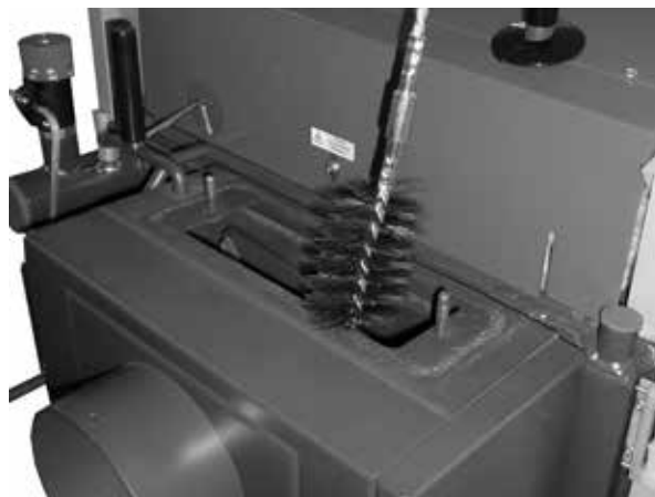
Sample cleaning of the smoke channel with a wire brush
