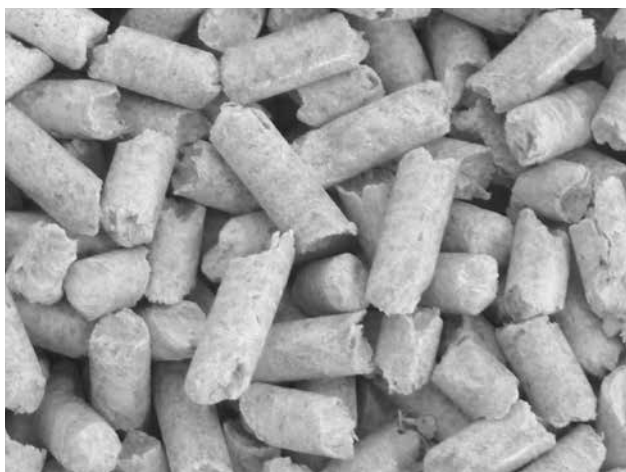
High-quality wooden pellets - white without black dots (bark)
