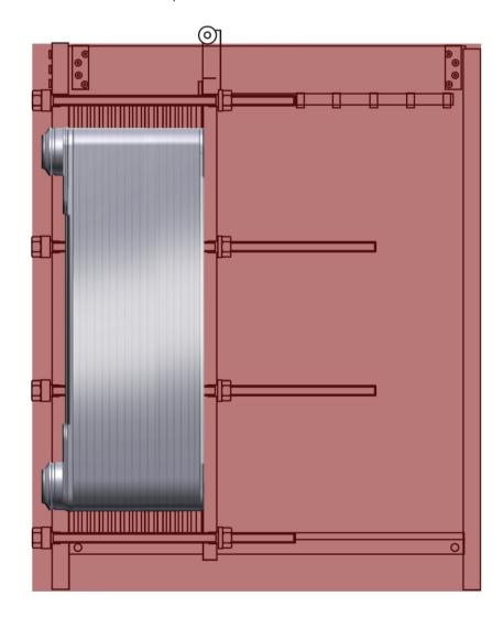
Installing a brazed plate heat exchanger leads to significant reductions in volume and weight, because gasketed plate heat exchangers of the same capacity require support equipment and pressure plates. The BPHE footprint is hence much smaller. This means great design freedom for every application - and reduced installation costs.
