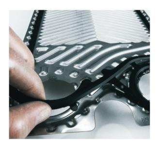
One of the main arguments for using PHEs instead of BPHEs is that PHEs can be taken apart and thoroughly cleaned. However, the process of chemically cleaning a PHE can be very expensive. The gaskets have to be removed prior to cleaning, and if they are glued to the plates (as many types of gaskets are), they have to be replaced at high cost with new ones after cleaning.
