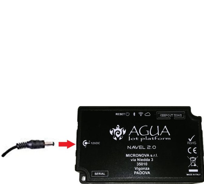
Figure 7. Power supply for Wi-Fi module
