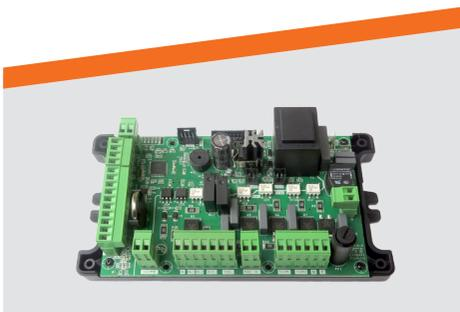
Regulation unit at every moment controls combustion. The control software adapts to the situation by providing at any time a minimum consumption of energy and optimal emission of gases.
