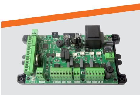
Regulation unit continuously controls combustion. The control software adjusts to provide minimum consumption of energy and optimal gas emissions.
