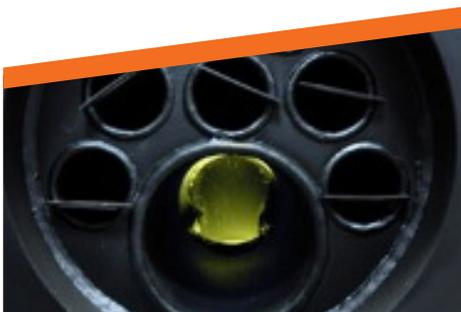
Tube heat exchanger is constructed with turbulators, which reduces the speed of exhaust gases, and also increases the surface area through which heat is transferred to water
